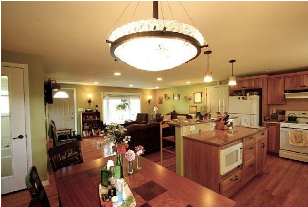
Open concept kitchen with Universal Design features: Level thresholds, 36-inch entryways, wide kitchen work aisle, rollout storage on the island, multiple height counters and an undercounter microwave oven.
